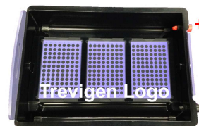
Figure 2: Assembling CometAssay ® ES for CometChip ® . Trevigen logo on CometChip ® adjacent to negative (black) electrode.
